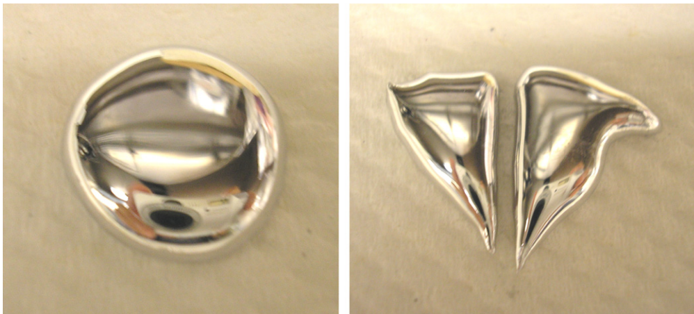
Fig. 6. Bead of pure Hg on the left assumes and maintains a roughly hemispherical shape despite probing with a plastic rod, while the same size bead of Hg–10 wt% In on the right has its shape readily manipulated. A plastic rod was dragged through the center of each bead just prior to this photograph. Actual bead size in each case was approximately 15 mm diameter.
